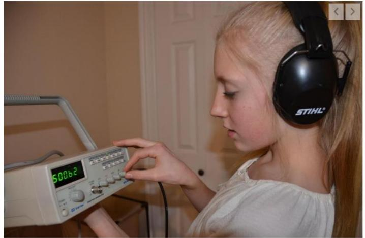
Oliva Washburn tests materials for sound attenuation value during the engineering phase of developing the Noisy NICU Cap.
